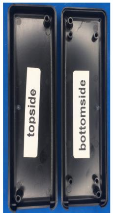
The bottom has 4 support points to fix the pcb.
