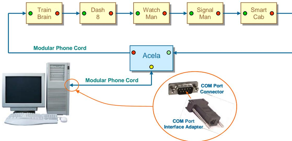
Figure 1-3 An Example of a COM Port-Connected Acela-Based CTI Network
