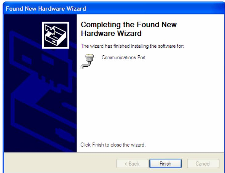
The Acela registers with Windows as a “virtual” COM port. This means that your application software can use the familiar (and easy-to-use) COM port programming model. You won’t need to worry about all the intricacies of USB interfacing.
