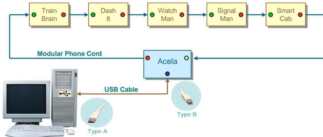
**Figure 1-4 An Example of a USB-Connected Acela-Based CTI Network**
