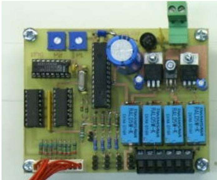
Figure 11: The MG V84 servo control interface
