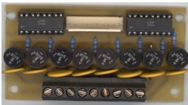
Figure 9: The MGV59 feed-back interface
